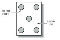
2FAM-C5R - Integrated Passive & Active Device using CSP
